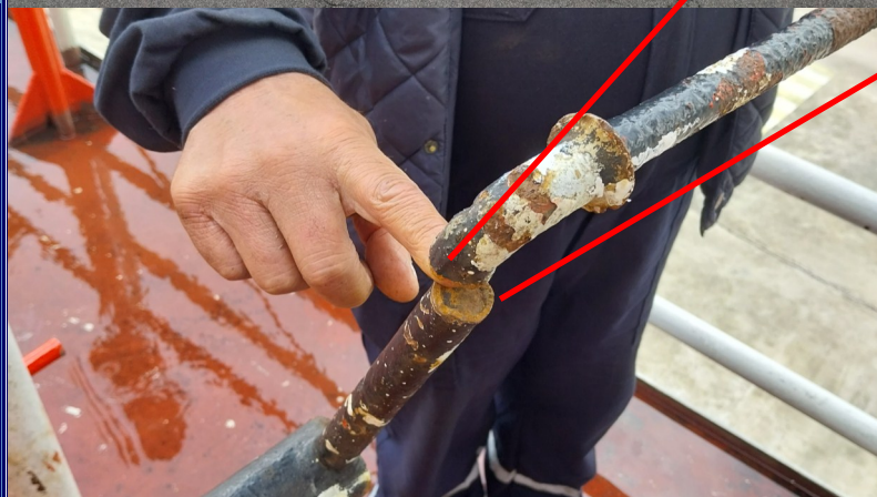
Figure2: The broken lever of the handle
